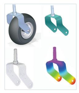
defining part to part boundary conditions, the edges of surfaces (from sheet metal mid-surfaces) can be glued to faces of other surfaces or solids, facilitating the simulation of more real-world scenarios. Since matching element sizing is no longer
